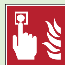
F005: Fire alarm call point
