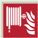
F002: Fire hose reel
