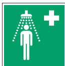
E012: Safety shower
