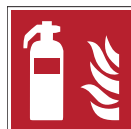
F001: Fire extinguisher
